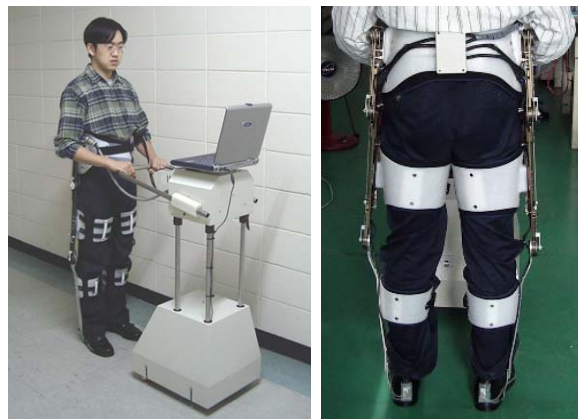
Fig. 1. Pictures of the tendon-driven exoskeletal power assistive device and caster walker
